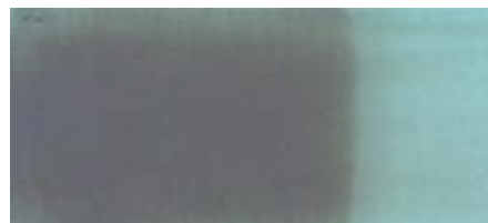
Figure 4. Photograph of the NiO film in the colored state (Left part of photo)
