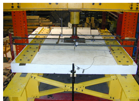
Fig. 3 Photo of one slab during testing
