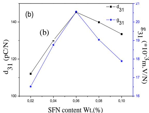
Fig. 5: SFN content Wt.(%) dependences of  $K_p$ ,  $Q_m$ ,  $d_{31}$ , and  $g_{31}$  for the (1-x)Pb(Zr<sub>0.53</sub>Ti<sub>0.47</sub>)O<sub>3</sub>-xSr(Fe<sub>2/3</sub>, Nb<sub>1/3</sub>)O<sub>3</sub> ceramics.
