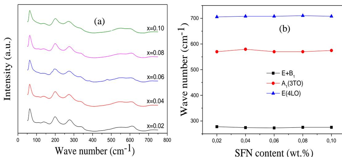
Fig. 3: Wave number (Raman shifts) of (a) various modes, and (b) E+B<sub>1</sub>, A<sub>1</sub>(3TO) and E(4LO) modes as a function of x content for  $(1-x)$ PZT- $x$ SFN ceramics.
