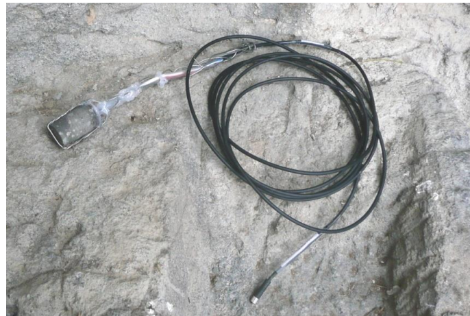
Figure 2. Moisture sensor with wire connections to RTM solar before inserting into rock massif.
