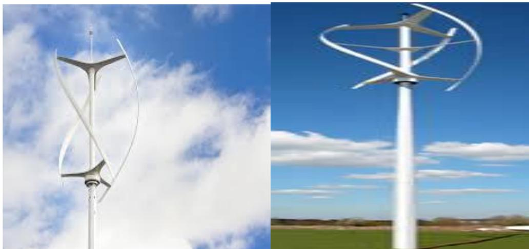
Figure I 2. Eolienne verticale.
