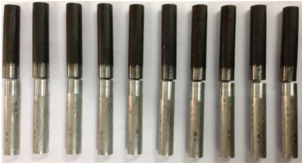
Figure 3. Macroscopic view of AA1100 aluminum alloy and mild steel specimens before welding
