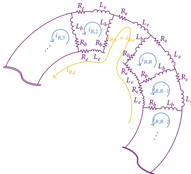
FIGURE 1 Squirrel cage IM equivalent circuit
