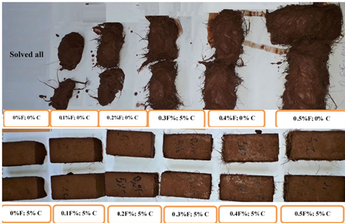
Fig. 13 Aspect of blocks after their immersion in water
