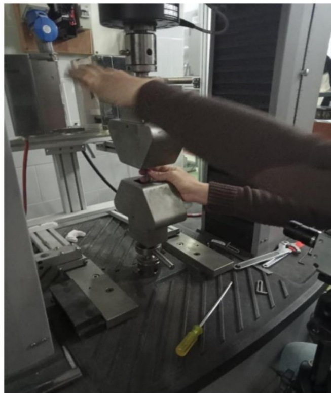
Figure II.4: Machine de traction (MTS Criterion TM model C45.105).
