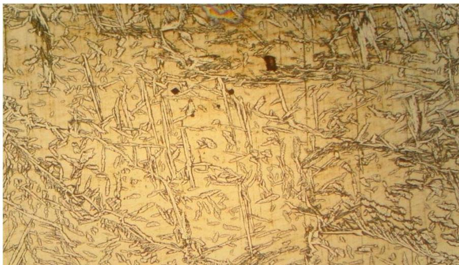
**Figure IV.4: Microstructure la ZAT de acier (2205).GX200**
