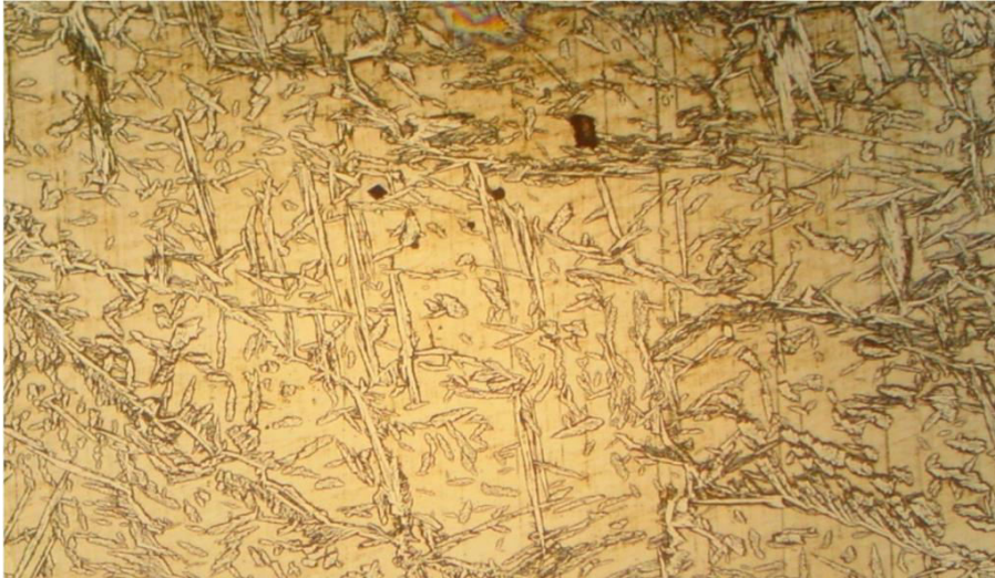
Figure IV.4: Microstructure la ZAT de acier (2205).GX200
