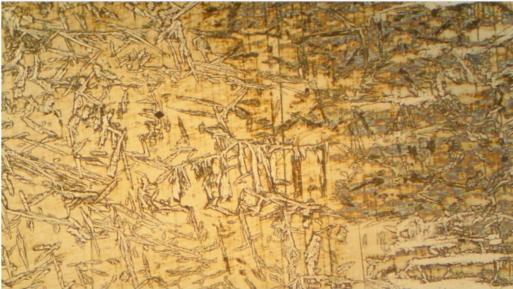
Figure IV.6 : Microstructure la ZL d'acier (2205) GX200
