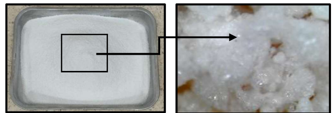
Fig. 2 Aspect of expanded perlite used
