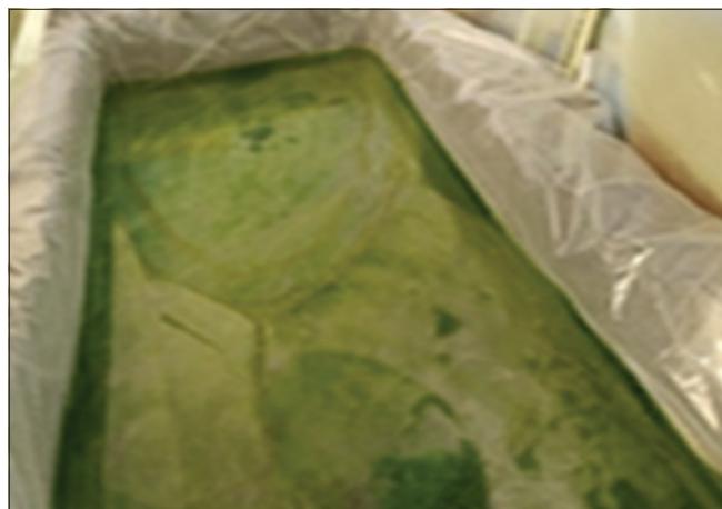
Fig 3. Basin (150 × 75 × 22 cm) of 180L just after the inoculation of the A. platensis .
