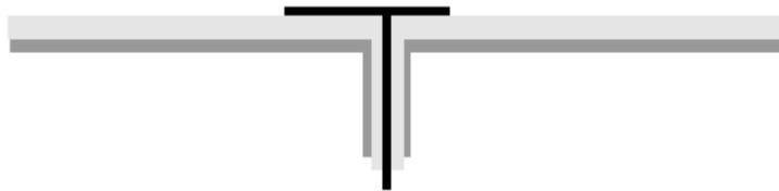
Figure II.10: patch antenna on a metal ground plane
