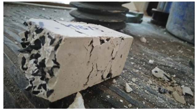
Fig. 10 Aspect of failed specimens
