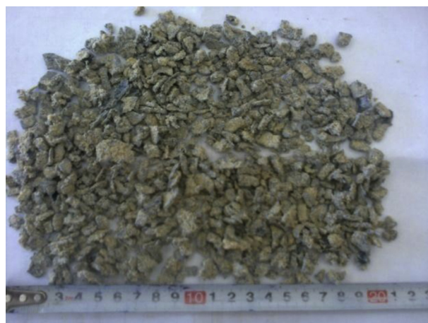
Fig. 3. Rubber treated with gluing-sand.
