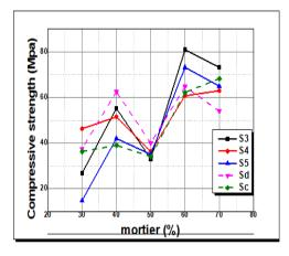
Figure 12. Variation of the compressive strength of concrete at 28 days according to the % of mortar
