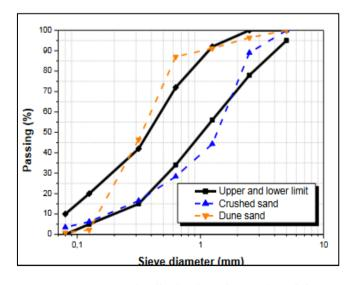
Figure 1. Granular distribution of SC and SD [4]
