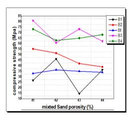
Figure 13. Effect of mixed sand porosity on the compressive strength at 28 days of the concrete
