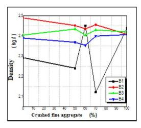
Figure 7. Density of the concretes according to the % of crushed sand
