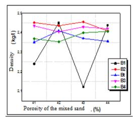
Figure 8. Density of the concretes according to the porosity of the mixed sand
