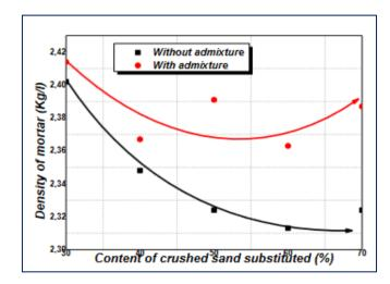
Figure 3. Density of mortars according to % of CS [4]
