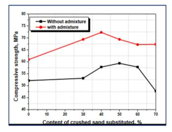
Figure 4. Compressive strength of mortars at 28 days according to the % of SC replaced [4]
