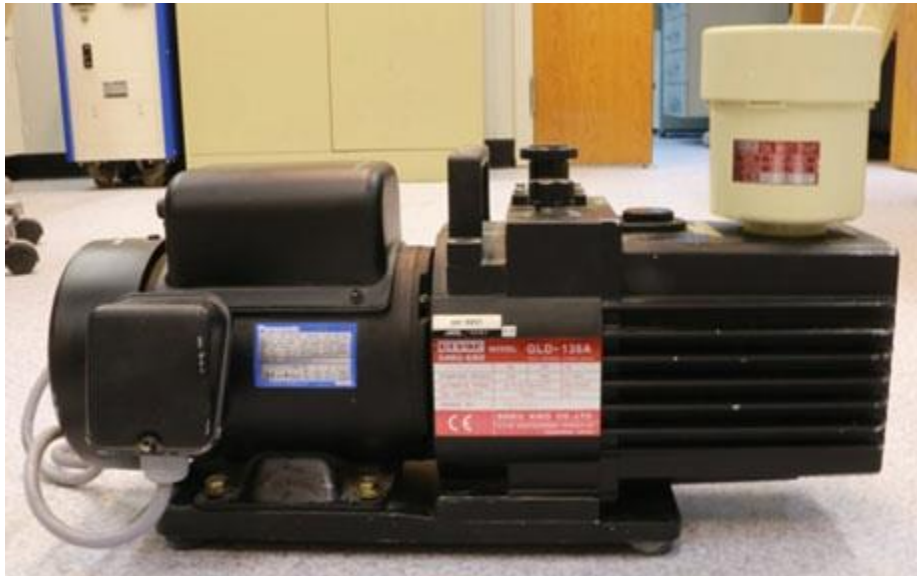
Figure II.3: of Common Rotary Pumps [3].
