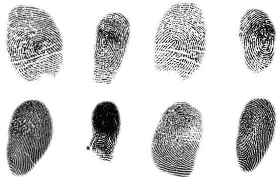
Fig. 1 Fingerprint images of LivDet 2023 database: top row (live samples), bottom row (fake samples). These samples are collected using Dermalog sensor.
