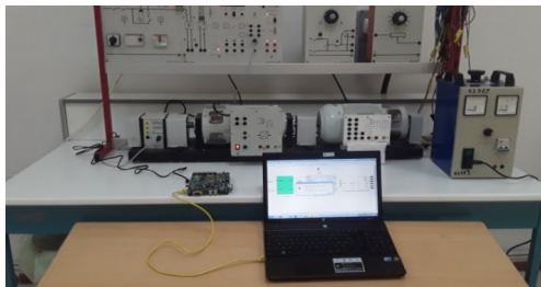
Fig. 11. Fuzzy DTC Point to Point Ethernet HIL process
