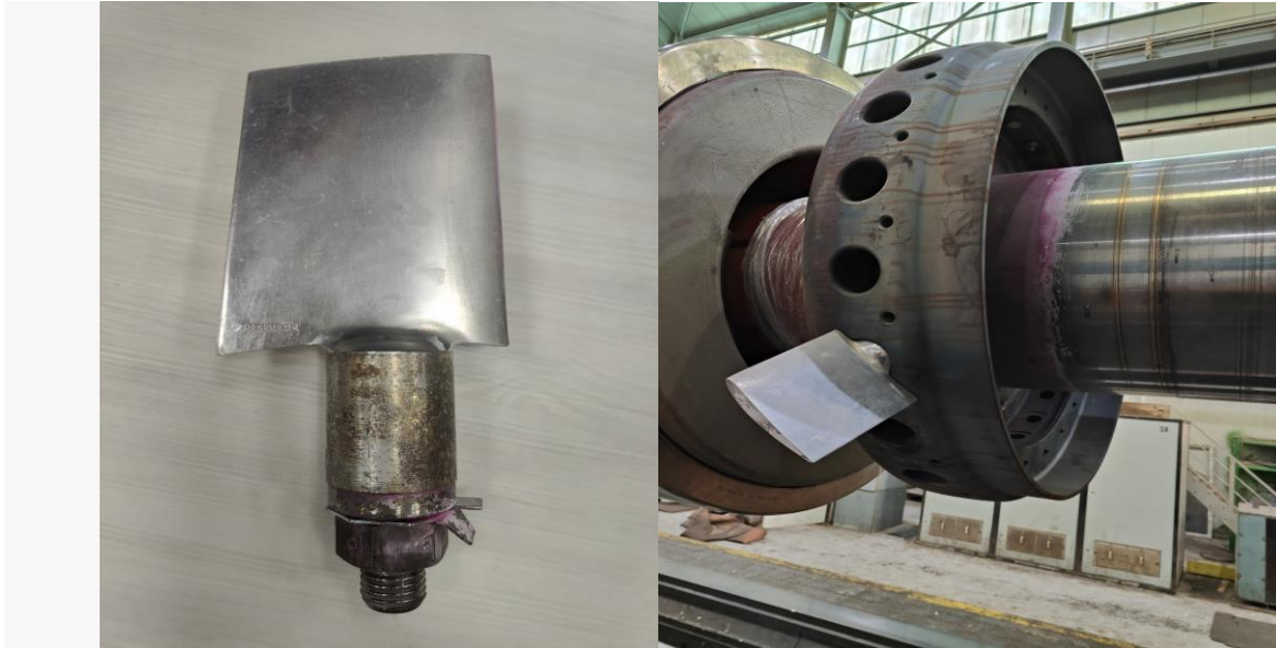
Figure I.1 : Rotary generator cooling blade and its installation location.
