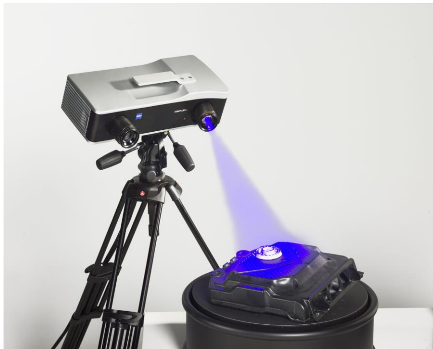
Figure III.2 : Scan of a mechanical part.
