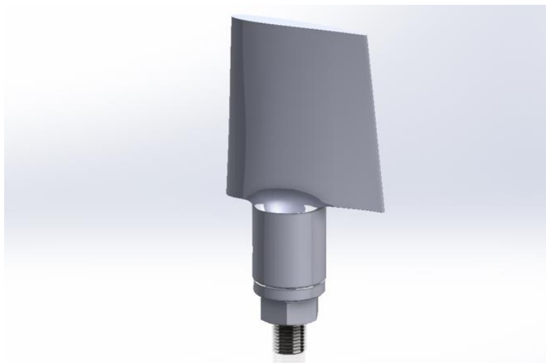
Figure III.11 : The final virtual Prototype for Rotary generator cooling blade.
