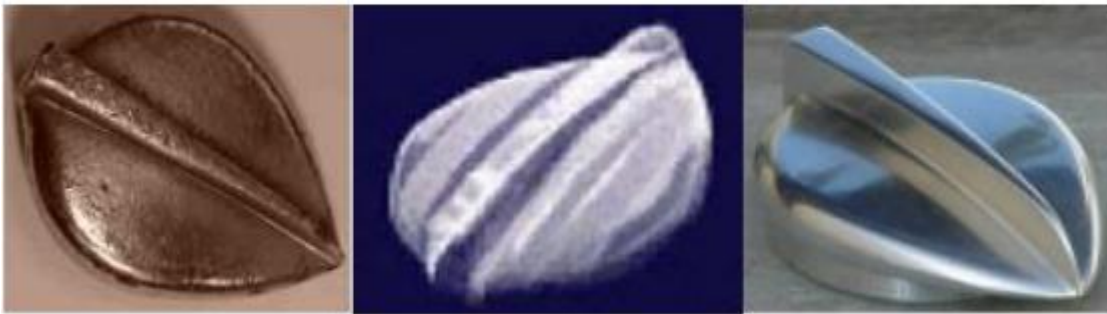
Figure II.5 : Reverse engineering of the car plug.
