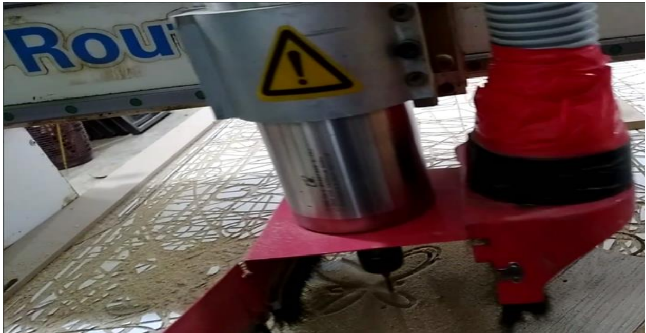
Fig. 2 Realization of the butterfly shape on a CNC machine
