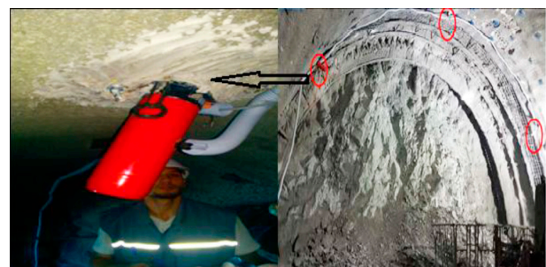
Fig. 4. Extensometer measurement system
