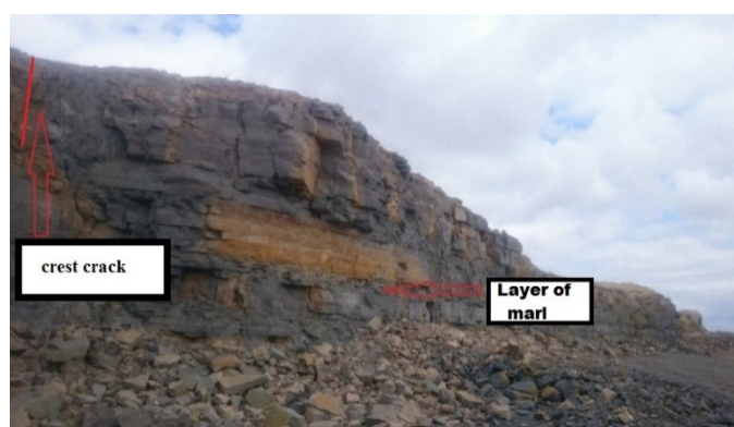
Fig. 3. Formation of the step at the level of the Chouf Amar quarry in the presence of a crest crack
