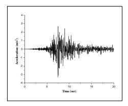
Fig. 4. Acceleration records of 2003 boumerdes earthquake.
