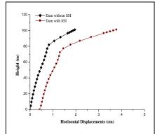
Fig. 5. Maximum horizontal displacements in upstream direction for model without SSI and model with SSI.
