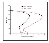
Fig. 10. Distribution of vertical stresses along dam height for model without SSI and model with SSI.
