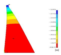
Fig.7. Maximum horizontal displacement contours of dam for model without SSI.
