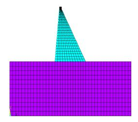
Fig. 3. Finite element model of dam-foundation rock system.
