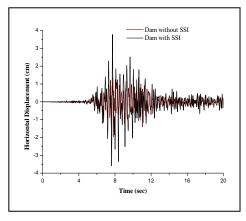
Fig. 6. Time history of horizontal displacement at crest of dam for model without SSI and model with SSI.
