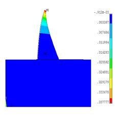
Fig. 8. Maximum horizontal displacement contours of dam for model with SSI.
