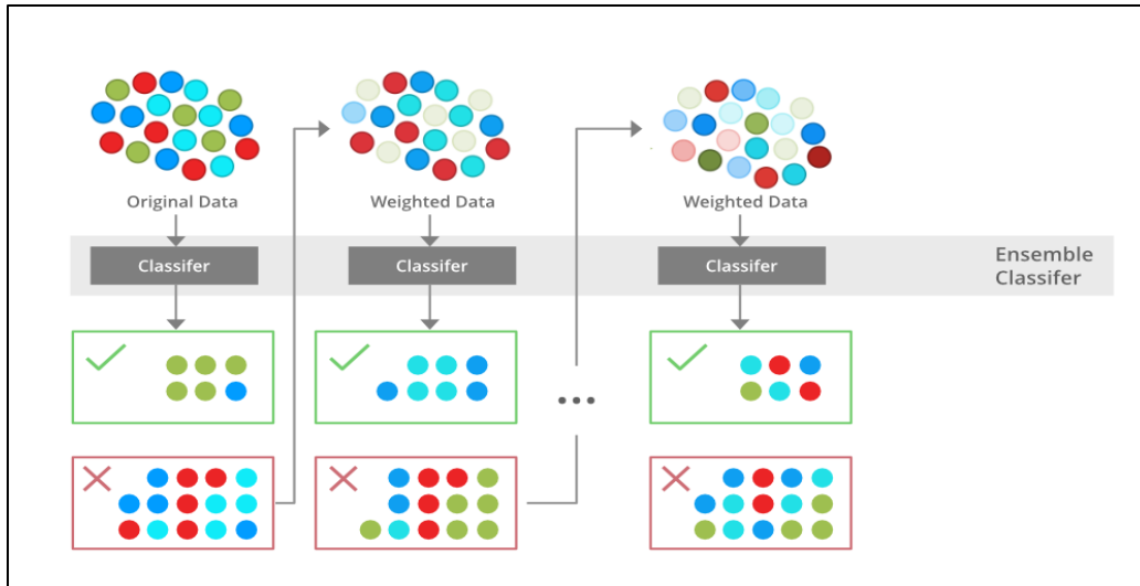
Figure 22. XGBoost Gradient Boosting schematic representation.
