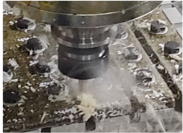
Fig. 12 Smoke emitted during slotting Alfa fibers composite
