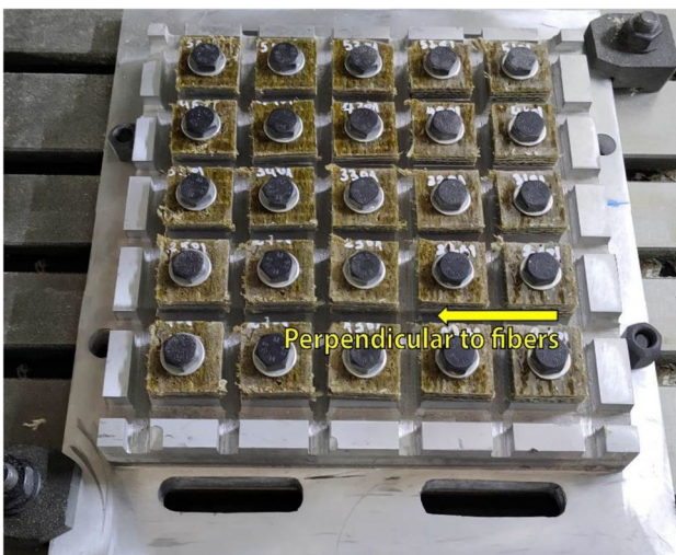
Fig. 11 Square coupons obtained by the trimming tests
