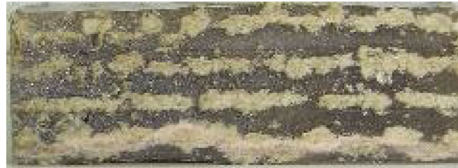
b) Down milling mode perpendicular to fiber, f=0.05\text{mm/rev} and v_c = 100\text{m/min}
