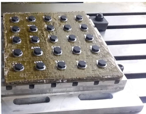
Fig. 5 Composite plate fixed in the machining fixture
