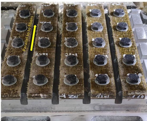
Fig. 10 Slotting parallels to fibers orientation
