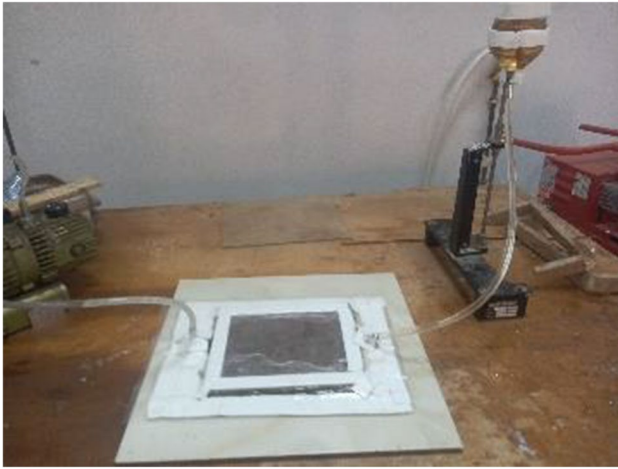
Fig. 1 Vacuum casting for producing composite plates
