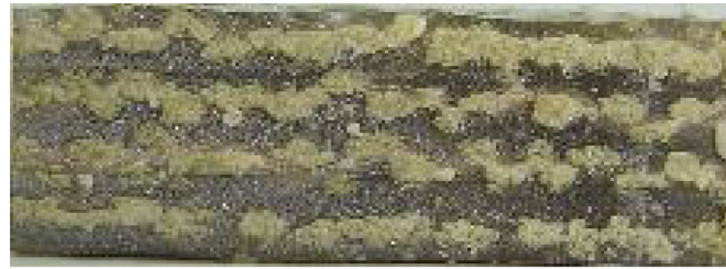
a) Up milling mode perpendicular to fiber, f=0.05\text{mm/rev} and v_c = 100\text{m/min}
