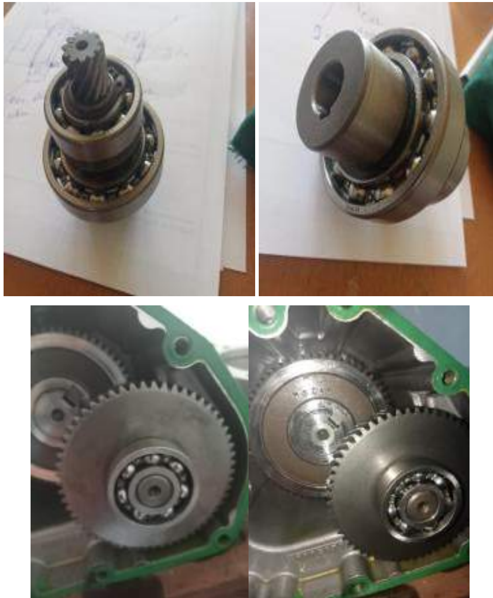
Fig. 6 Inner components: rotating shaft, bearing and helicoidal gears
