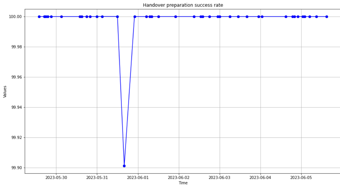
Figure IV.7: KPI Handover preparation success rate in the cell 283004.
