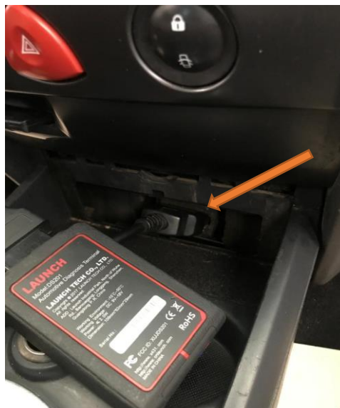
Figure IV. 12: branchement du scanner launch
