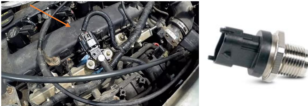
Figure III. 7: capteur pression carburant
