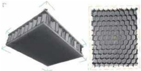
Fig.1: Honeycomb sandwich structure with face-sheet and the honeycomb core
