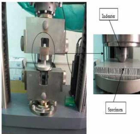
Fig. 2: The test system used in the quasi-static indentation tests (Zwick/Roell).
