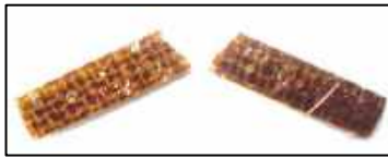
Fig. 10. Example of a test piece damaged in impact
