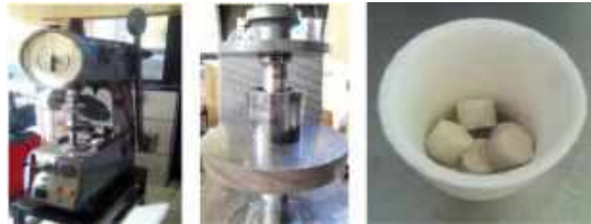
Fig. 2. Vertical hydraulic press and tools used to compress the powder mixture.
