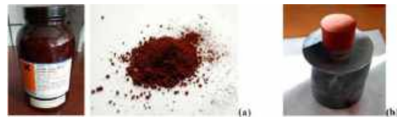
Fig. 5. (a): Images of the used ferric oxide (hematite) (b): A pressed pellet before melting.
