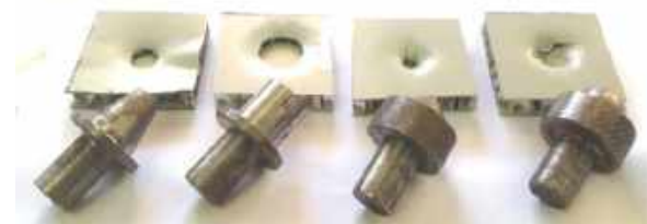
Figure 6 : Failure modes observed during indentation: failure of face: (skin/core debonding, fracture of the
