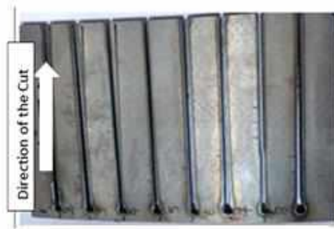
Figure 1 Plasma arc cut specimens
