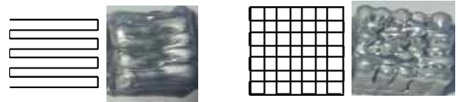
Fig. 5. Filling strategies for massive parts
