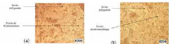
Fig.7. melt zone microstructure of welded sheet metal at speeds (a) 16mm/s and (b) 8 mm/s GX200
