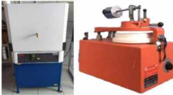
Fig. 6. Secondary melting electric furnace and mortar grinder utilized.
