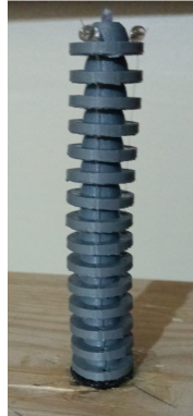
Fig. 5.9: A section of the continuum robot design with a novel ball disk [19]
