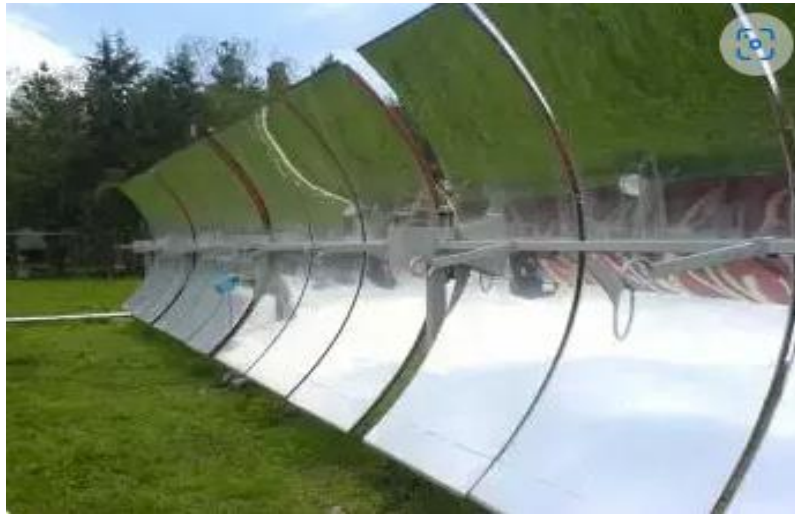
Figure.I.12. Parabolic trough collectors[19]
