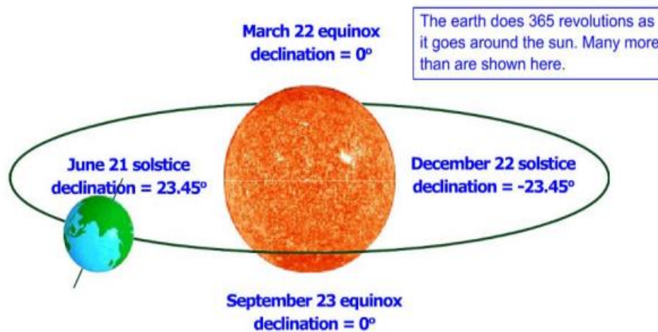
Figure I.3. declination angle for one year. [11]
