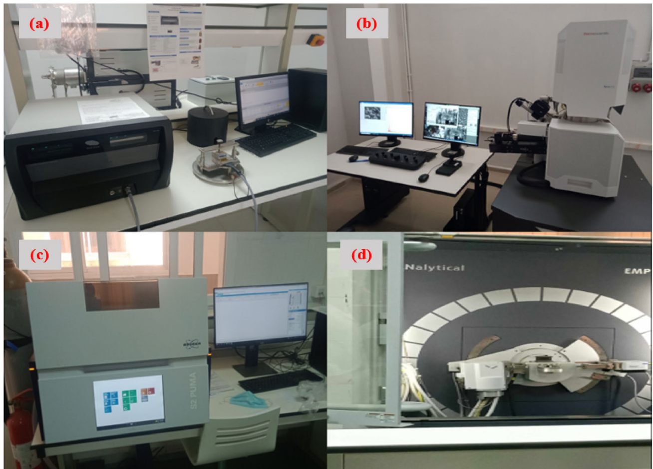
Fig. 6 Equipment used for analyzing the thermal properties and microstructure of the samples a Hot Disk test b SEM test c XRF test d XRD test
