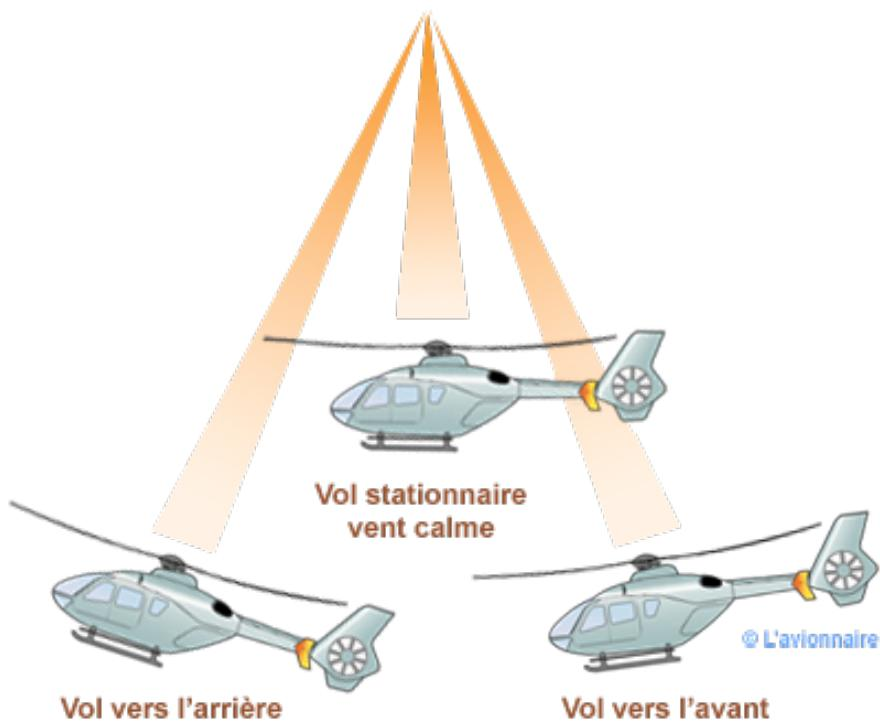
figure II 5 : Pendulum Motion of the Helicopter Fuselage
