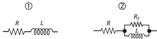
Figure 2-18: Equivalent diagrams of a coil
