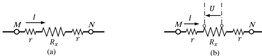
Figure 2-11: (a) Equivalent diagram of a real resistor (b) Four-terminal resistor
