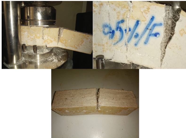
Figure 6. Fracture surface of Typha angustifolia fiber-reinforced plaster composite after failure.
