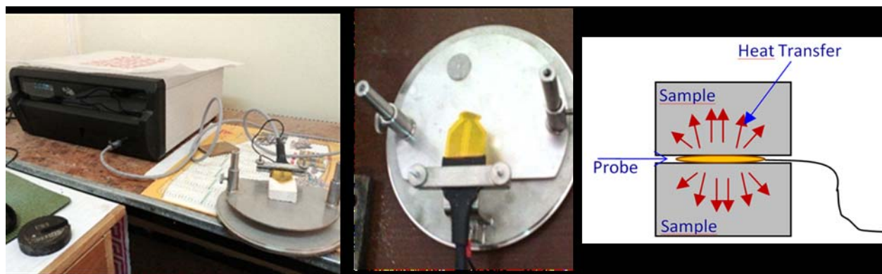
Fig. 4. Experimental setup used for the measurement of the thermal properties.
