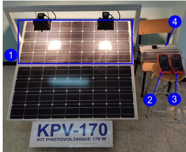
Fig. 2. The STP085B-12 Solar photovoltaic panel. (1): Panel, (2): Amperemeter, (3): Voltmeter, (4): Load.
