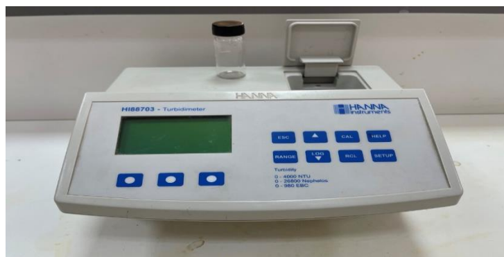
Figure I.12: Turbidimètre Hanna "HI88703"
