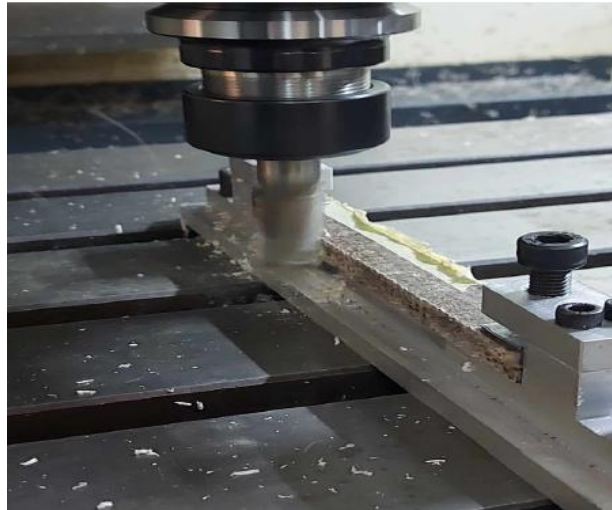
Fig. 12. Execution of the specimen machining program
