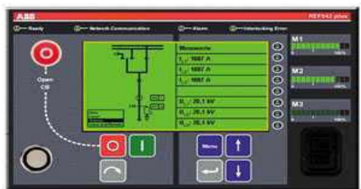
Figure 3.8 The HMI Control Unit
