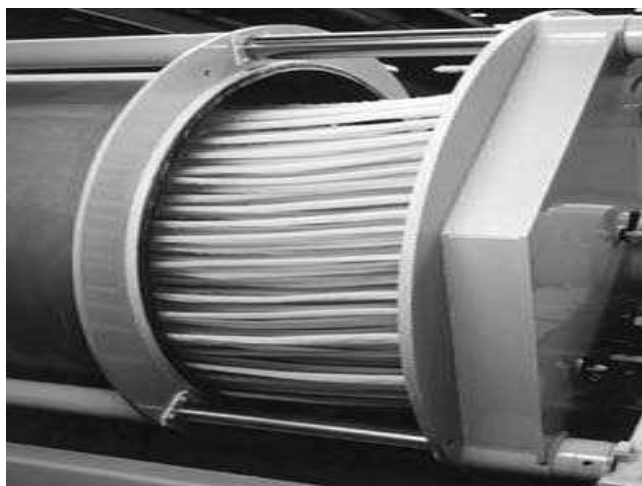
Figure II.2. Pressoir rotatif horizontal : Pressoir à fruits universel HP5000 (Bucher-Guyer)
