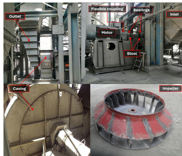
Fig. 1 Pictures of the section where the FN280 centrifugal fan is placed in the plant with pictures of the impeller
